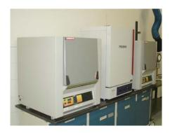
MTF 12/38/250/201 single zone solid tube furnace, Heated length of 250MM, Maximum temperature 1200°C, (Qty. 6)
